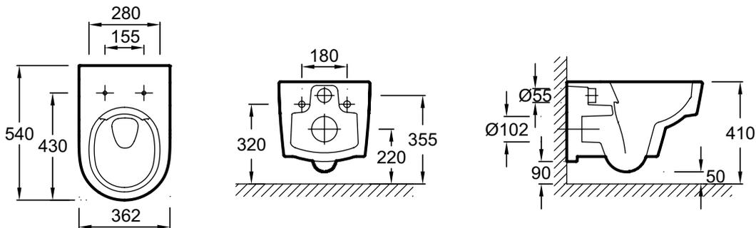
Product Specification: Rimless wall-hung WC pack. EDR112. Collection: ODÉON RIVE GAUCHE. DIMENSIONS: 54 x 36.20 cm. WEIGHT: 23.4 kg. MATERIAL: Ceramic. INSTALLATION TYPE: Wall-hung. NORMS AND REGULATION: NF. VOLUME OF WATER: 2.6/4 L and 3/6 L. HEIGHT: Comfort. RIM TYPE: Rimless. RIM: Without rim. PRODUCT INCLUDED: (seat included). SEAT : Included. TOILET BOWL FIXINGS: Invisible.
