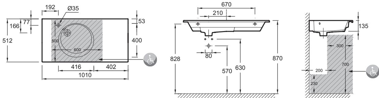
Product Specification: Vanity top 100 cm. EXAU112. Collection: ODÉON RIVE GAUCHE. DIMENSIONS: 101 x 51.20 cm. WEIGHT: 28.4 kg. MATERIAL: Ceramic. INSTALLATION TYPE: Self-supporting. TAP DRILLING: 1 tap hole. GROUND/UNGROUND: Without ground underside. OVERFLOW: With. NUMBER OF VANITY BASINS FOR VANITY TOPS: Single basin. RECOMMENDED TAPS: Odéon Rive Gauche (several finish options).
