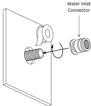
Apply thread tape (or similar) to the ½" connection, then screw the top rail connector to the connection.
