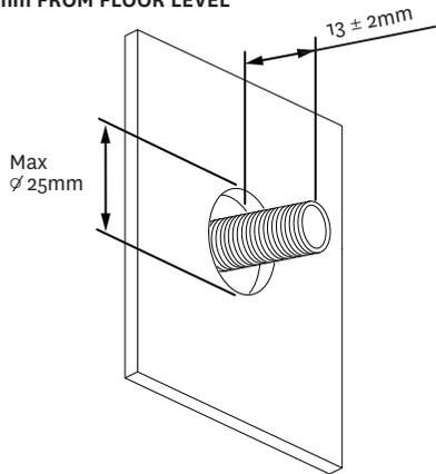
Install a ½" male threaded connection at the recommended height on wall, ensuring that a minimum of 10mm of thread protrudes past the finished wall.
