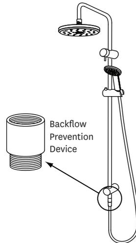
Make sure a washer is in both ends of the hose. Screw hose onto lower outlet on wet rail, attach handset and place firmly in holder. Tilt and rotate head to the desired position.
