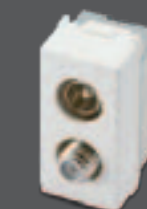
FDDBS-21277-18 Coaxial TV/RD/SAT 5-2400 Mhz socket outlet, through-line connection, with 2 IEC 60169-2 male and female connector, 18db attenuation Presse coassiale IEC-F Mas-Fem passante dB 18 Toma coaxial IEC-F Macho-Hembra de paso dB 18
