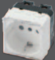
FDBS-21174 2P+E 16A, P30, 250V~ Shuko socket outlet with transparent cover, Italian standard Presa UNEL P30 2P+T laterale e centrale Base de enchufe UNEL
