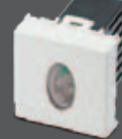
FDDBS-21465.2 Emergency light with white LED, 16cd luminous intensity, 120 minutes duration, 230V~ Lampada d'emergenza 2 moduli, autonomia 120', luminosità 16cd, alimentazione 230V~ Lampara de emergencia, autonomía 120', luminosidad 16cd
