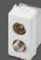
FDDBS-21277-14 Coaxial TV/RD/SAT 5-2400 Mhz socket outlet, through-line connection, with 2 IEC 60169-2 male and female connector, 14db attenuation Presse coassiale IEC-F Mas-Fem passante dB 14 Toma coaxial IEC-F Macho-Hembra de paso dB 14
