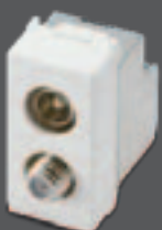
FDDBS-21277-7 Coaxial TV/RD/SAT 5-2400 Mhz socket outlet, through-line connection, with 2 IEC 60169-2 male and female connector, 7db attenuation Presse coassiale IEC-F Mas-Fem passante dB 7 Toma coaxial IEC-F Macho-Hembra de paso dB 7
