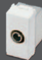
FDDBS-21270-DC Coaxial TV/RD/SAT 5-2400 Mhz socket outlet, through-line connection, with IEC 60169-2 male connector, 18db attenuation Presse coassiale IEC Maschio diretta 5-2400Mhz con passaggio di corrente Toma coaxial IEC Macho directa 5-2400Mhz con paso de corriente
