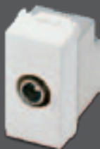
FDDBS-21270-7 Coaxial TV/RD/SAT 5-2400 Mhz socket outlet, direct connection, with IEC 60169-2 male connector, allows DC current passage Presse coassiale IEC Maschio passante dB 7 Toma coaxial IEC Macho de paso dB 7
