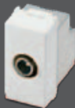
FDDBS-21270-10 Coaxial TV/RD/SAT 5-2400 Mhz socket outlet, through-line connection, with IEC 60169-2 male connector, 7db attenuation Presse coassiale IEC Maschio passante dB 10 Toma coaxial IEC Macho de paso dB 10
