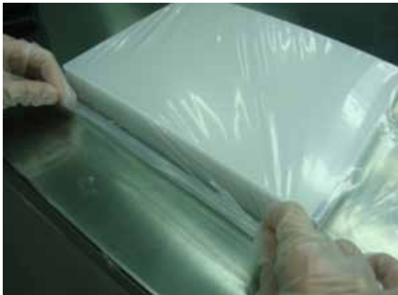
Image 1b (Folding wrapping along height of stack)
